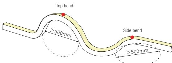
Note: Min bending diameter of Top bend>500mm,
