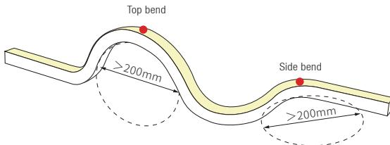
Note: Min bending diameter of Top bend>200mm,
